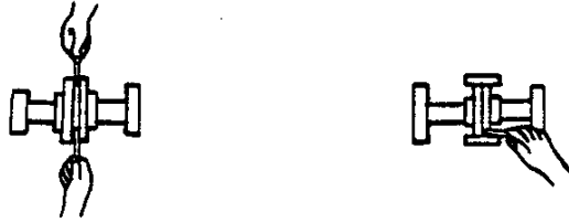
Figure 3b. Aligning Non-Spider Type Couplings
