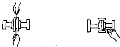
Figure 3B. Aligning Non-Spider Type Couplings
