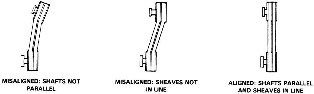
Figure 7. Alignment of V-Belt Driven Pumps
