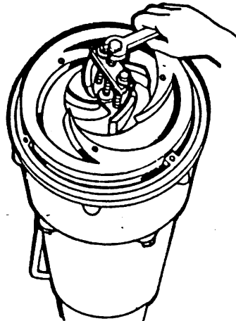
Figure 2. Removing Impeller With Puller
