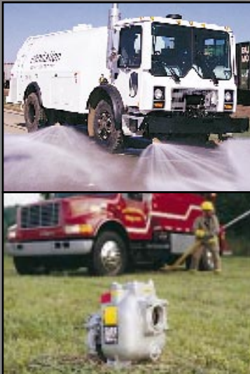
0 Series® high-pressure, self-priming centrifugal pump is mounted on a fire truck for direct pumping from the tank to the fire in Ohio, USA.
