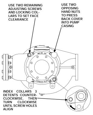
Figure C--6. Installing and Adjusting Back Cover
