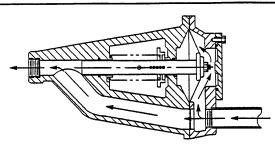
Figure 1. Valve in Open Position
