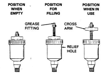
Figure 3. Automatic Lubricating Grease Cup
