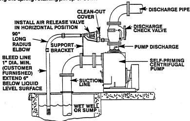
Figure 3. Typical Automatic Air Release Valve Installation
