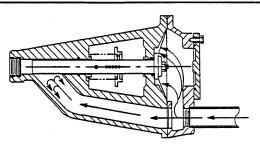
Figure 2. Valve in Closed Position
