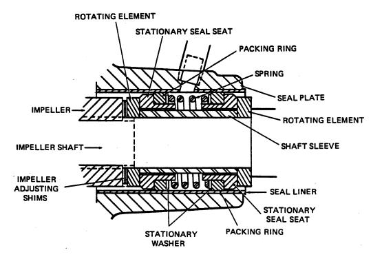
Figure 2. GS01500 Seal Assembly
