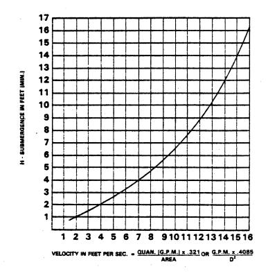
Figure 2. Recommended Minimum Suction Line Submergence Vs. Velocity
