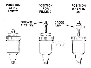
Figure 5. Automatic Lubricating Grease Cup
