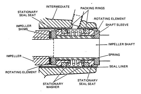
Figure 4. GS-1500 Seal Assembly
