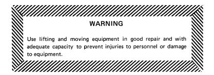
Make sure that hoists and other lifting equipment are of sufficient capacity to safely handle the pump assembly. If chains and cables are used, make certain that they are positioned so that they will not damage the pump, and so that the load will be balanced.
