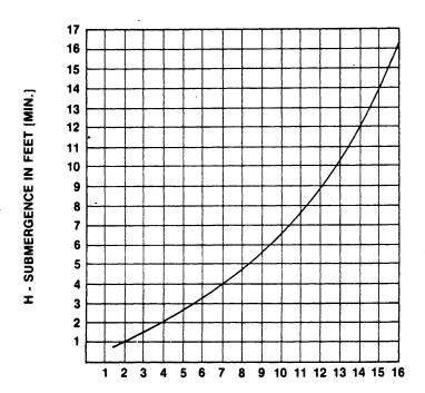
VELOCITY IN FEET PER SEC. =  $\frac{\text{QUAN. [G.P.M.]} \times .321}{\text{ARFA}}$  OR  $\frac{\text{G.P.M.} \times .4085}{\text{D}^2}$
