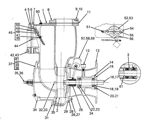
Figure 3. Pump End Only Model 16A2
