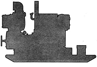
The only moving parts of this pump are the impeller, seal rotating elements, and the shaft. The wear plate, impeller, and seal, which receive the most wear, are easily accessible and can be replaced without disturbing the piping. Maintenance and replacement of these three parts will maintain the peak operating efficiency of the pump.
