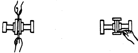
Figure 3B. Aligning Non-Spider Type Couplings
