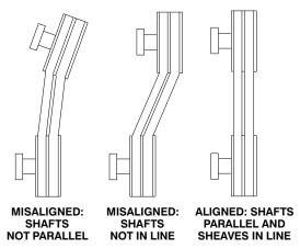
Figure 3C. Alignment of V-Belt Driven Pumps
