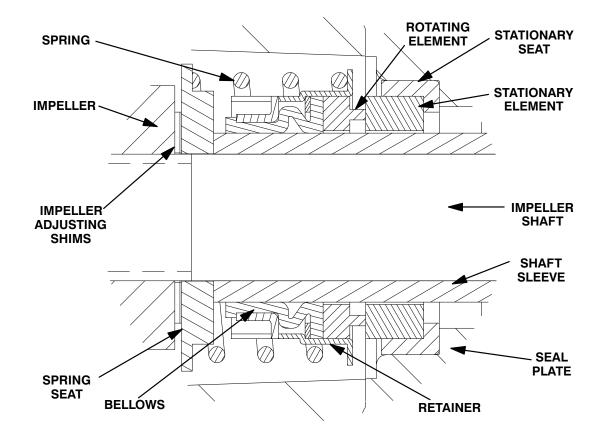
Figure 3. Seal Assembly
