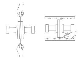
Figure 3B. Aligning Non-Spider Type Couplings
