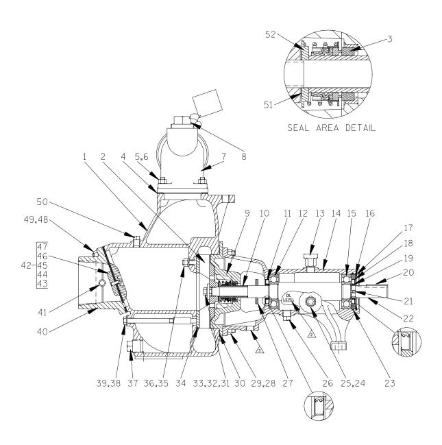
Figure 1. Pump Model 83A3-B
