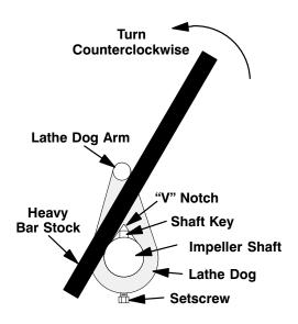
Figure 2. Loosening Impeller
