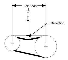
Figure 4. Belt Tension Measurement
