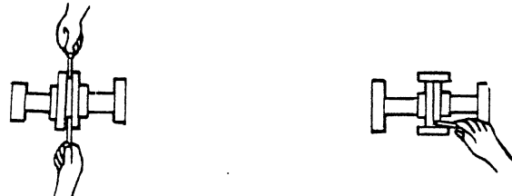
Figure 5A. Aligning Non-Spider Type Couplings
