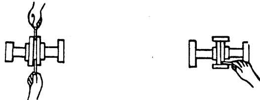
Figure 5A. Aligning Non-Spider Type Couplings
