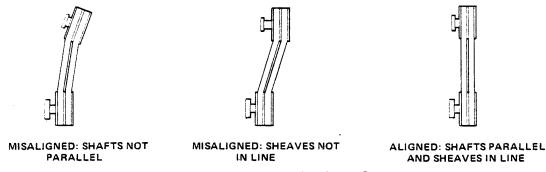
Figure 5C. Alignment of V-Belt Driven Pumps
