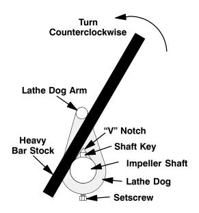
Figure 3. Loosening Impeller
