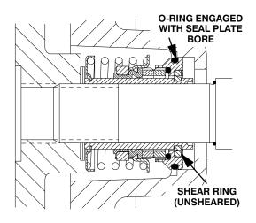
Figure 6. Seal Partially Installed
