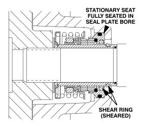
Figure 7. Seal Fully Installed
