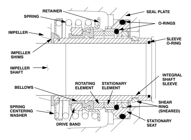
Figure 5. Cartridge Seal Assembly
