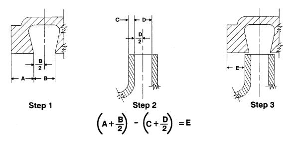
Figure 4. Centering Impeller Within Pump Casing
