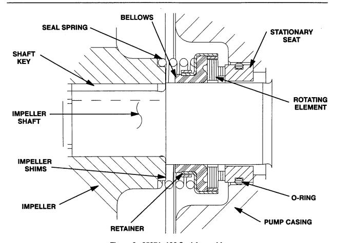
Figure 2. 25271-192 Seal Assembly
