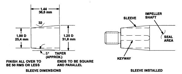
Figure 3. Seal Installation Sleeve
