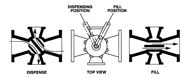
Figure 5. FDF Valve Theory of Operation
