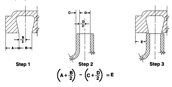
Figure 4. Centering Impeller Within Pump Casing
