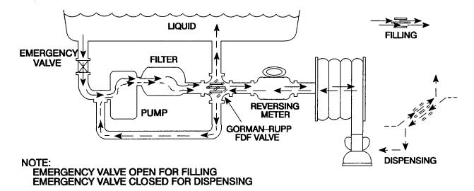
Figure 4. Typical Installation Using Pump For Filling And Dispensing
