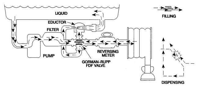
Figure 3. Typical System Installation Using Educator For Filling And Dispensing
