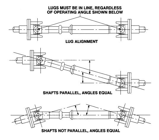
Figure 2. Proper Installation And Alignment of Universal Assembly
