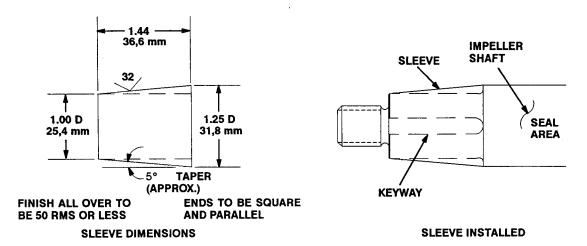
Figure 3. Seal Installation Sleeve
