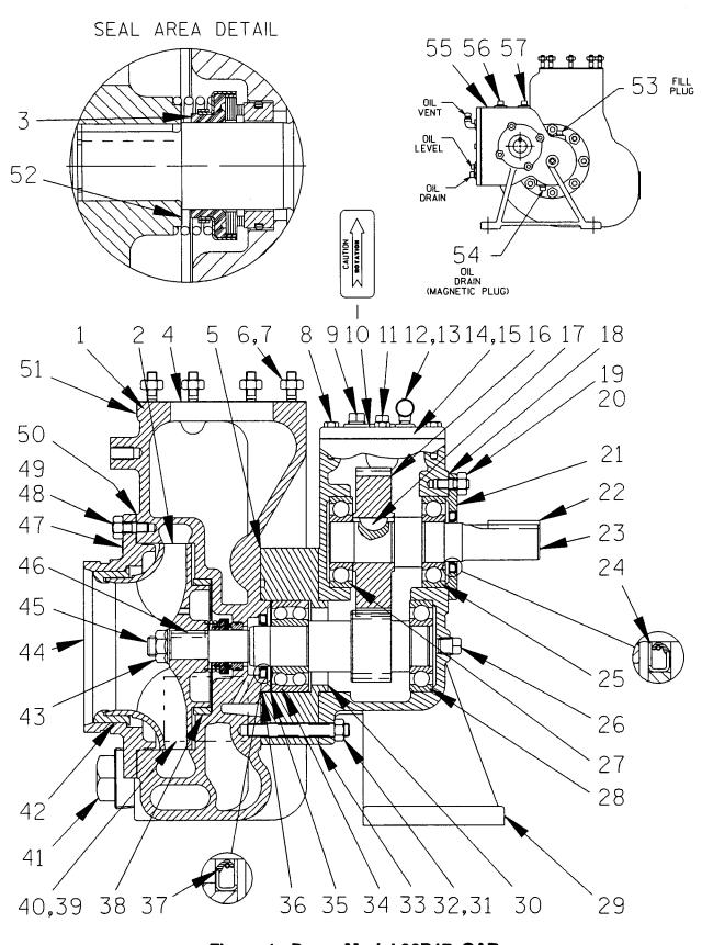
Figure 1. Pump Model 06D17-GAR
