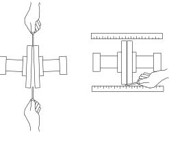
Figure 3B. Aligning Non-Spider Type Couplings
