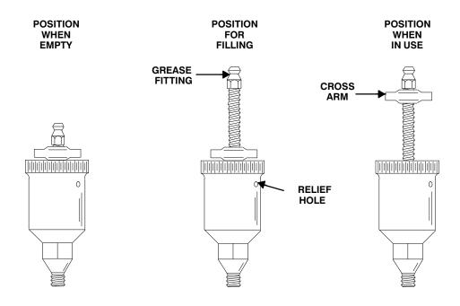
Figure 4. Automatic Lubricating Grease Cup
