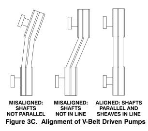
Tighten the belts in accordance with the belt manufacturer's instructions. If the belts are too loose, they will slip; if the belts are too tight, there will be excessive power loss and possible bearing failure. Select pulleys that will match the proper speed ratio; overspeeding the pump may damage both pump and power source.
