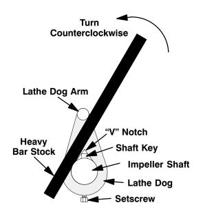
Figure 2. Loosening Impeller
