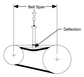
Figure 4. Belt Tension Measurement
