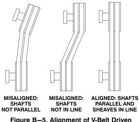
Figure B-5. Alignment of V-Belt Driven
