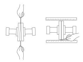
Figure B-4. Aligning Non-Spider-Type Couplings
