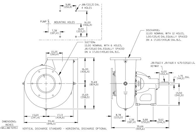
Figure B-1. Pump Model 612L20B-B
