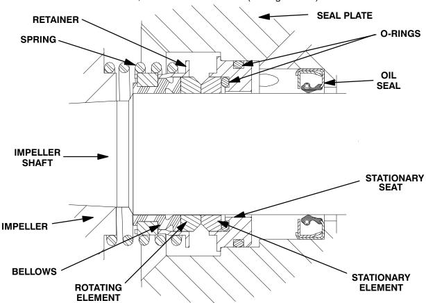
Figure E-4. 12590B Seal Assembly
