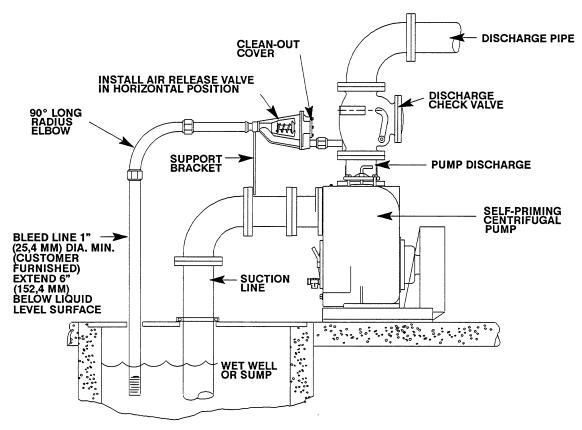
Figure 5. Typical Automatic Air Release Valve Installation
