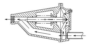
Figure 3. Valve in Open Position
