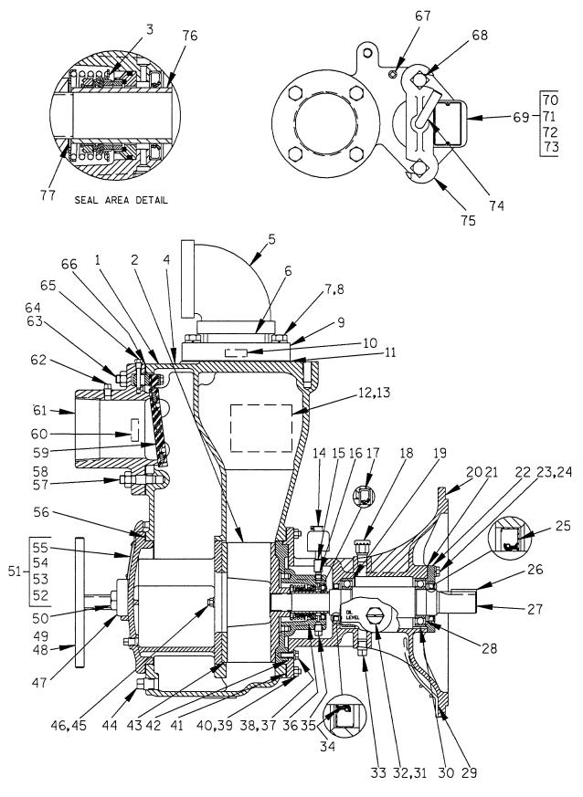
Figure 2. 14C20-(SAE 4/10) Pump End Assembly
