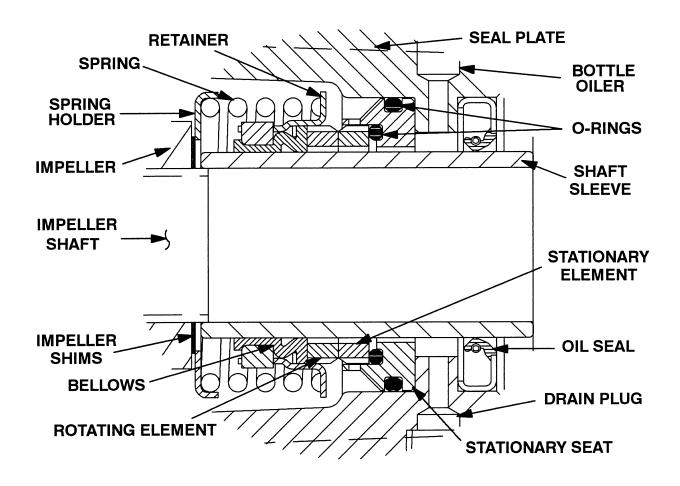
Figure 4. 12364D Seal Assembly
