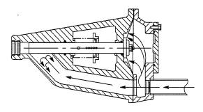
Figure 4. Valve in Closed Position
