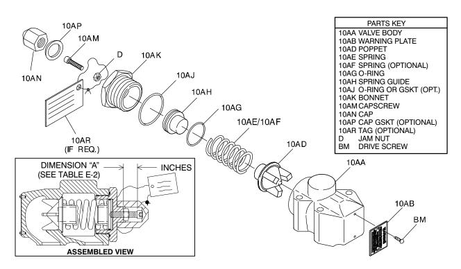
Figure E-6. Pressure Relief Valve Assembly
