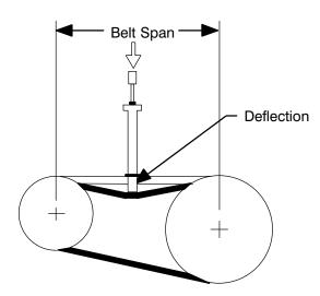
Figure B-5. Belt Tension Measurement
