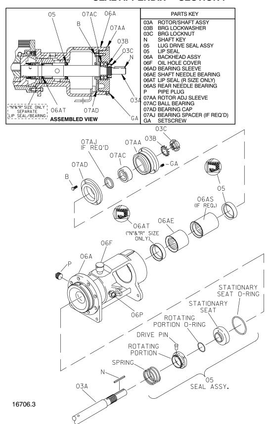
Figure F-2. Lug Drive (Option 62A And 62B) Mechanical Seals
