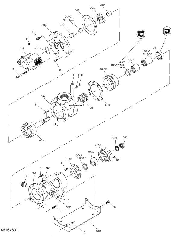
**Shown:** Standard Model With 90° Ports, Head-Mounted Relief Valve and Optional Foot Bracket. Also Available With 180° Ports And/Or Head Jacket, Housing-Mounted Relief Valve. A Coverplate Kit Replaces Either Relief Valve When Not Used.
