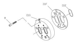
Figure E-2. Typical Head Jacket Assembly
