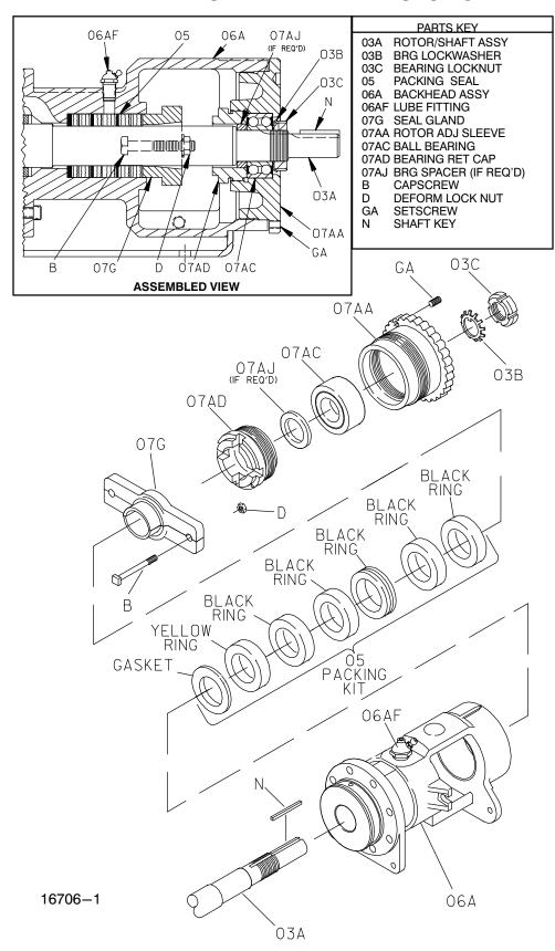
Figure F-3. Minimum Leak Packing Seal (Option 65S)
