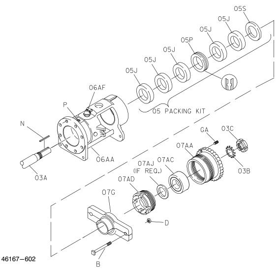
Figure F-4. Standard Packing Seal (Option 65)
