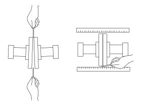
Figure B-3. Aligning Non-Spider Type Coupling
