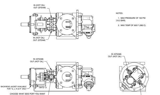
Figure H-1. Inlet / Outlet Location
