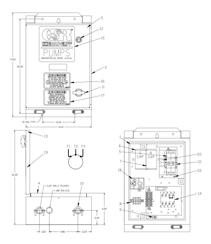
Figure 2. 27511-105 NEMA Type 3R Control Box Dimension
