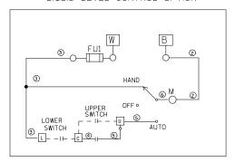
Figure B-6. Control Box 27511-105 Elementary Wiring Diagram
