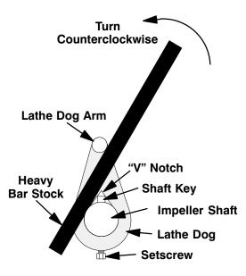
Figure 3. Loosening Impeller
