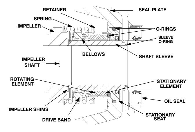
Figure 6. Cartridge Seal Assembly
