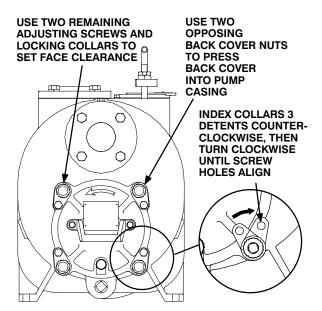
Figure 9. Installing and Adjusting Back Cover
