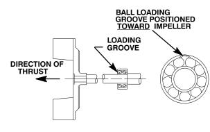
INSTALLATION OF MRC/SKF 5300M OR FAFNIR 5300W SERIES BEARINGS (OPEN OR ENCLOSED IMPELLERS)
