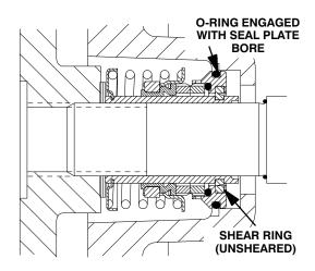
Figure 7. Seal Partially Installed
