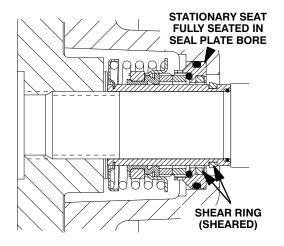
Figure 8. Seal Fully Installed
