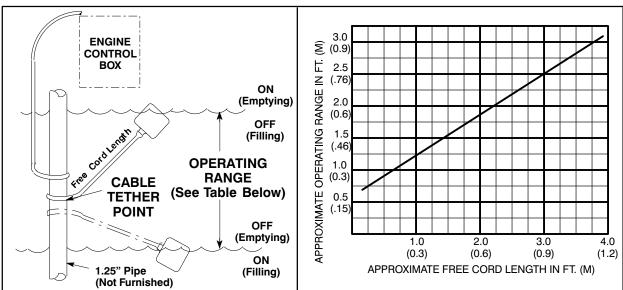
Figure 3. Float Switch Data
