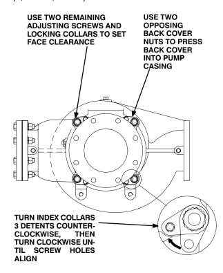
Figure 11. Installing and Adjusting Back Cover
