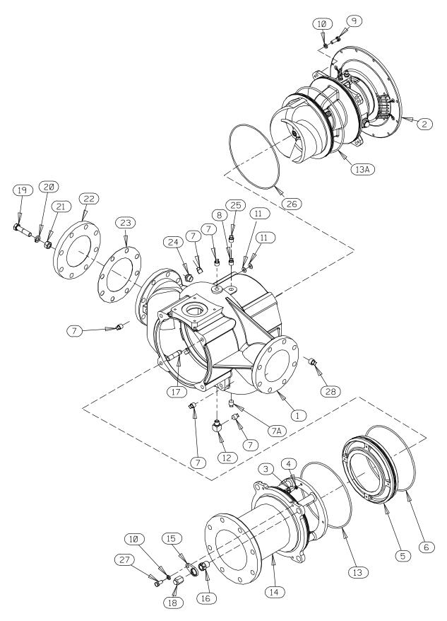
Figure 4. PA6C60-(4045H) Pump Subassembly
