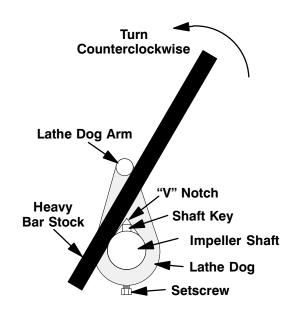
Figure 9. Loosening Impeller
