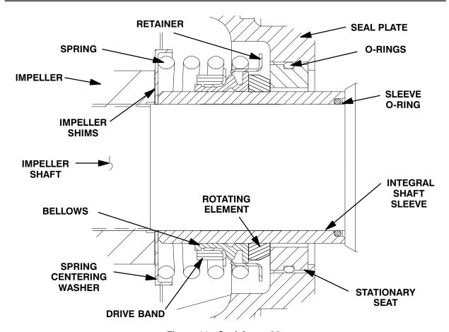
Figure 10. Seal Assembly
