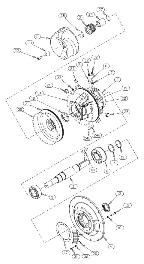
Figure 5. 44163-502 Repair Rotating Assembly
