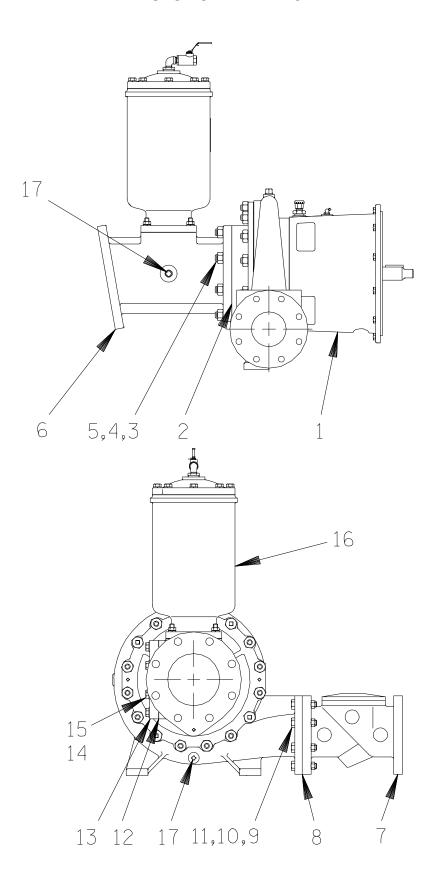
Figure 3. PA4B60-(SAE 4/10) Pump End Assembly
