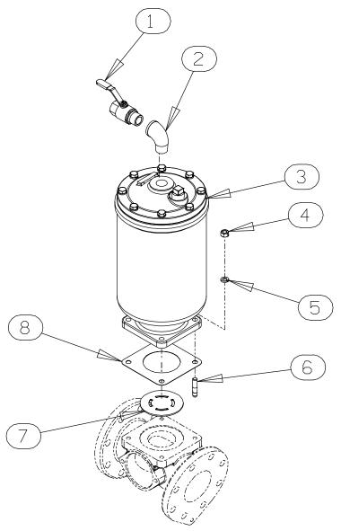
Figure 6. 48275-006 Priming Chamber Kit
