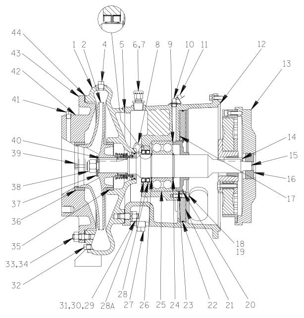
Figure 4. 64B60-(SAE 4/10) Pump Assembly
