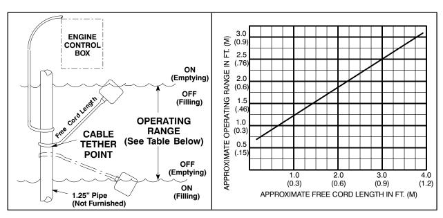
Figure 3. Float Switch Data
