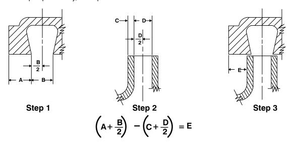
Figure 10. Centering Impeller Within Volute Scroll
