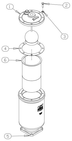
Figure 7. 46112—709 Priming Chamber Assembly
