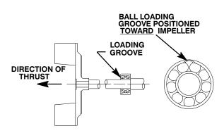
INSTALLATION OF MRC/SKF 5300M OR FAFNIR 5300W SERIES BEARINGS (OPEN OR ENCLOSED IMPELLERS)
