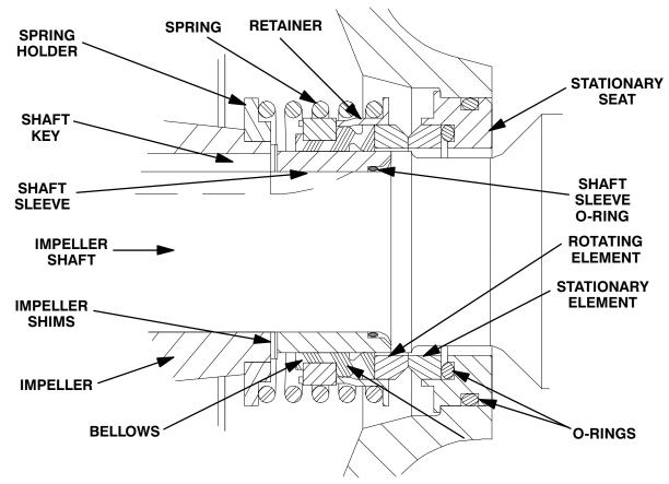
Figure 9. 46512-048 Seal Assembly
