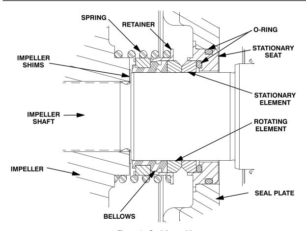
Figure 9. Seal Assembly
