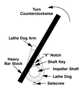
Figure 8. Loosening Impeller
