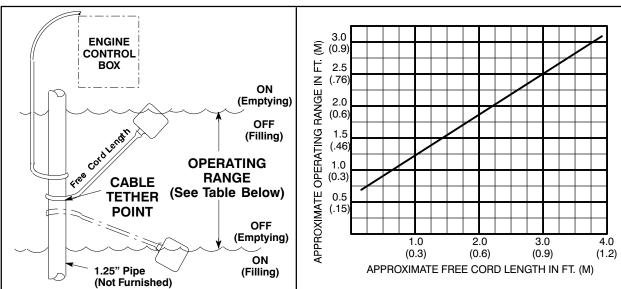
Figure 3. Float Switch Data
