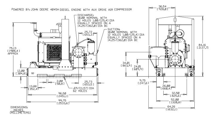
Figure 1. Pump Model PA10A60-4045H
