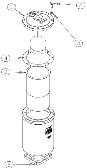
Figure 6. 46112—709 Priming Chamber Assembly
