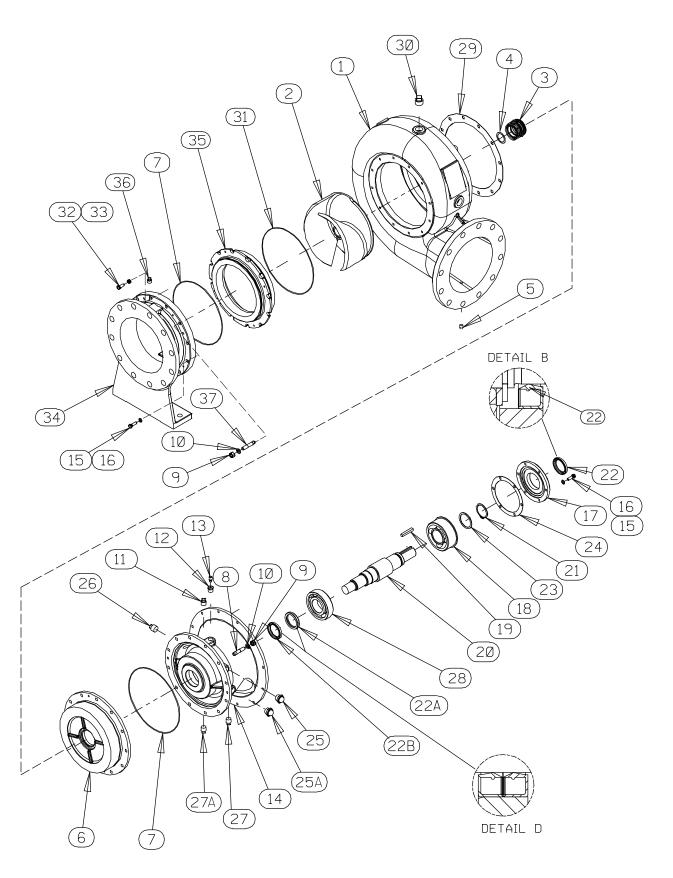
Figure 4. 610N60-(SAE 3/11.5) Pump End Assembly
