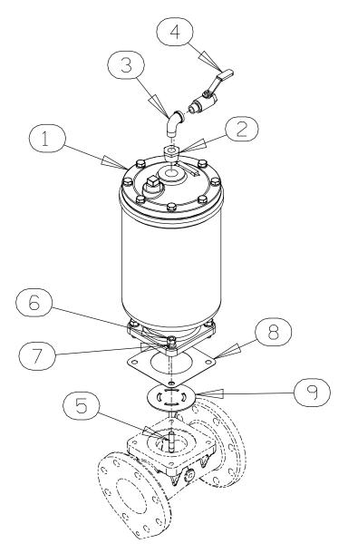
Figure 5. 48275-005 Priming Chamber Kit
