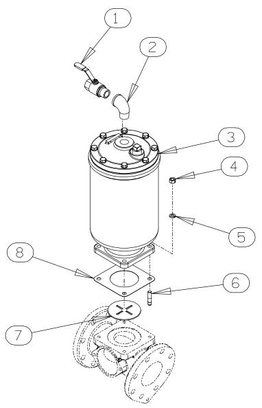
Figure 6. Priming Chamber Kit
