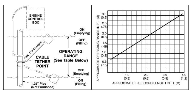
Figure 3. Float Switch Data
