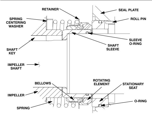
Figure 10. Seal Assembly
