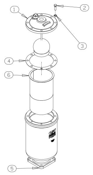
Figure 7. Priming Chamber Assembly
