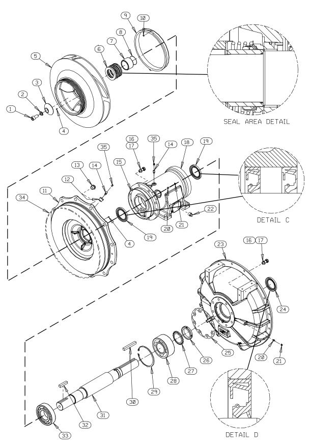
Figure 5. Repair Rotating Assembly
