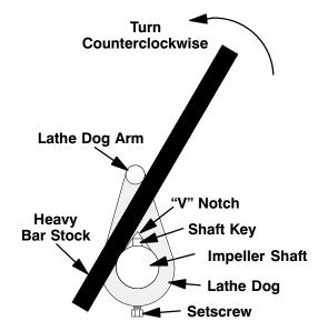
Figure 9. Loosening Impeller
