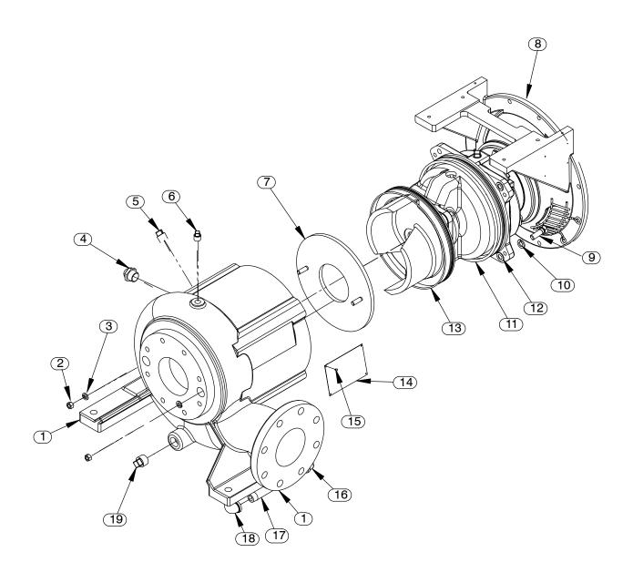
Figure 4. Pump End Assembly
