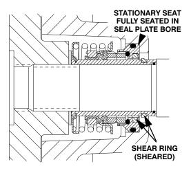
Figure 13. Seal Fully Installed
