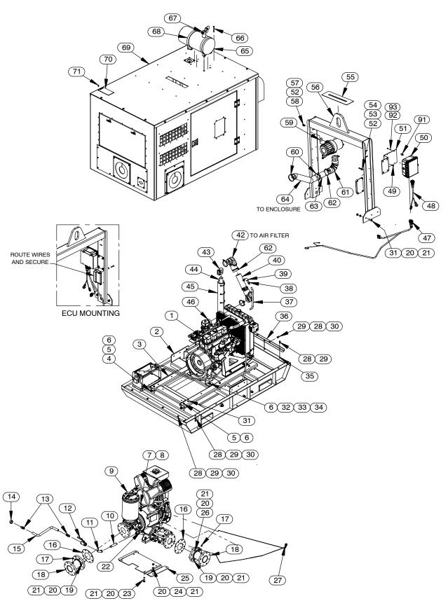
Figure 1. Pump Model PA4A60C-ZPP428-ESP
