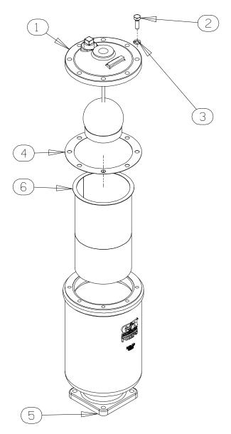
Figure 7. Priming Chamber Assembly PARTS LIST
