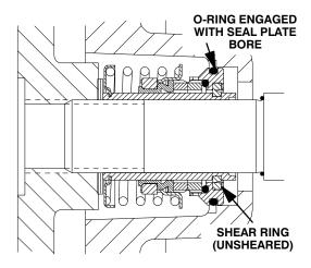
Figure 12. Seal Partially Installed
