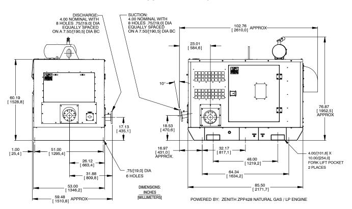
Figure 1. Pump Model PA4A60C—ZPP428—ESP
