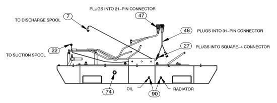
Figure 2. Pump Model PA4A60C-ZPP428-ESP (cont'd)
