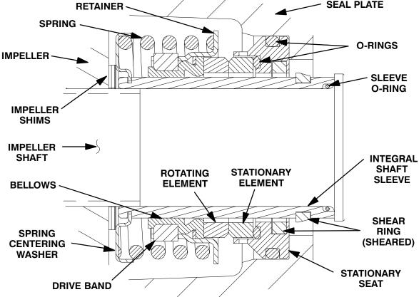
Figure 11. Cartridge Seal Assembly
