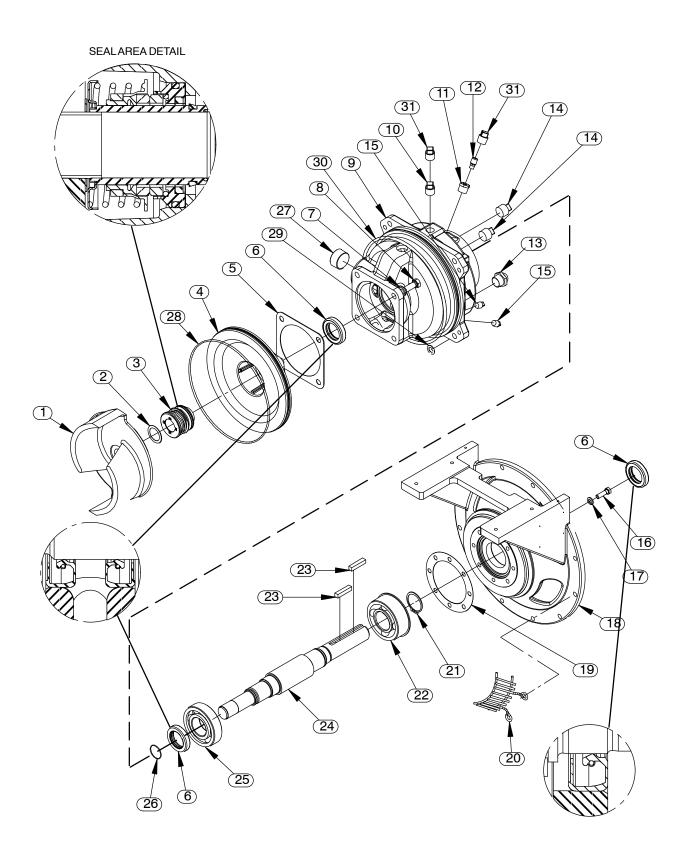
Figure 5. Repair Rotating Assembly
