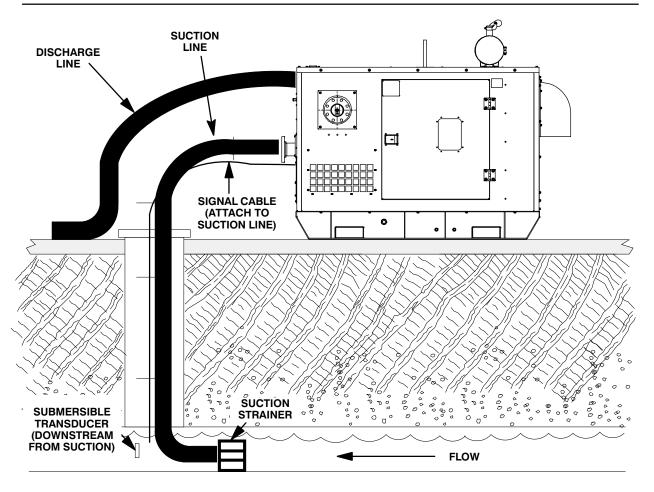
Figure 3. Typical Submersible Transducer Installation
