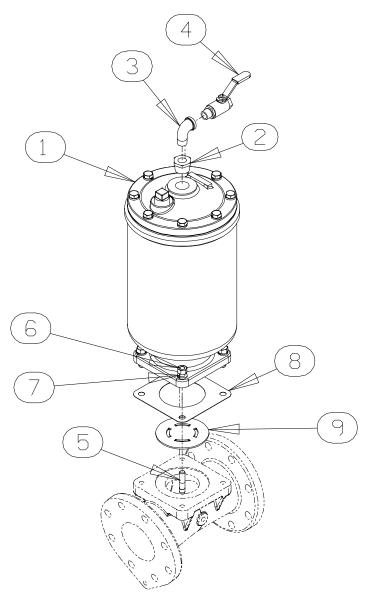
Figure 6. Priming Chamber Kit
