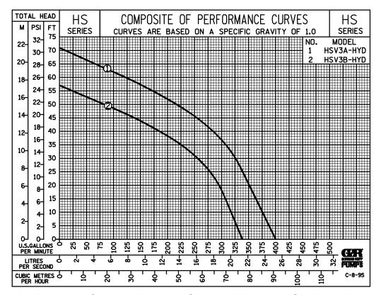
Performance Curve — Models HSV3A1—HYD And HSV3B31—HYD
