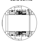
Seal: Mechanical; Self-Lubricated. Fluorocarbon Elastomers (DuPont Viton® or Equivalent). Carbon Rotating Face; Ni-Resist Stationary Face; Maximum Temperature of Liquid Pumped is 160°F (71°C).\*
