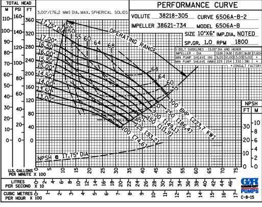
**60 HERTZ PERFORMANCE BASED ON** WATER **TRIMMED IMPELLER**
