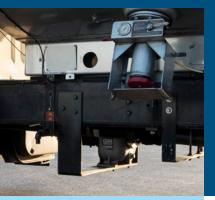
Gorman-Rupp selfpriming centrifugal Power Take-Off Pumps are ideal for handling aircraft fuels, fuel oil, gasoline and other petroleum derivitives.
