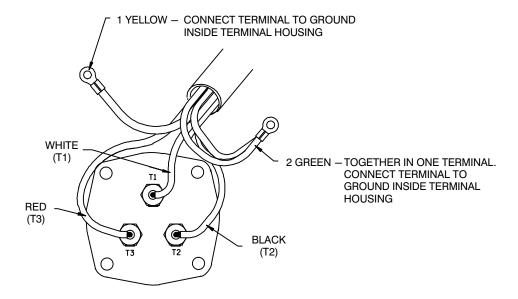
Figure C-7. Terminal Housing Wiring Connections
