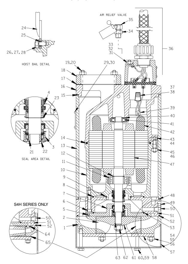
Figure C-1. Typical S4C, S4D And S4H Series Pump Assembly
