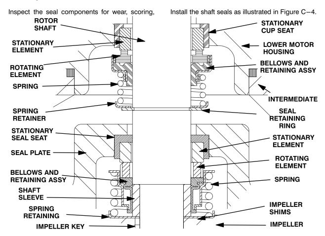
Figure C-4. Upper And Lower Seal Assemblies
