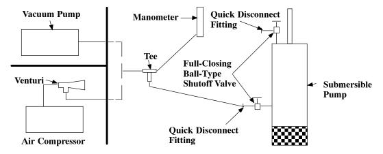
Figure C-8. Vacuum Test System
