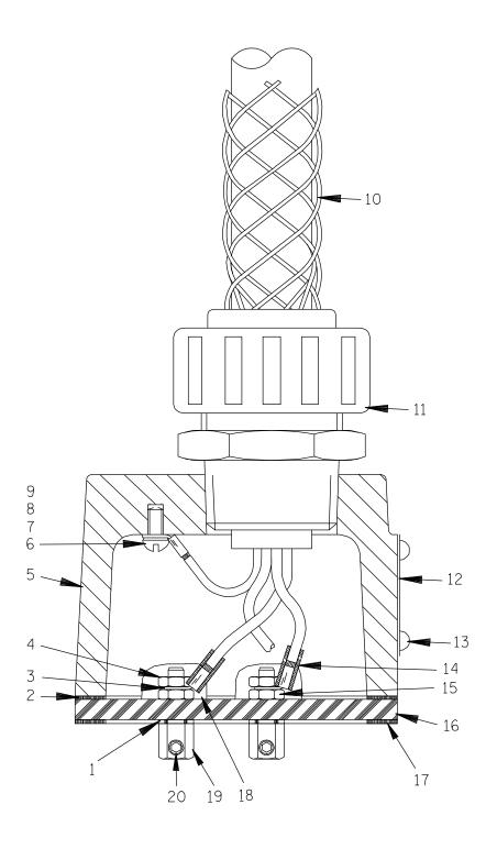
Figure C-2. S4C,S4D And S4H Terminal Housing And Cable Assembly Standard and SST-Fitted Models
