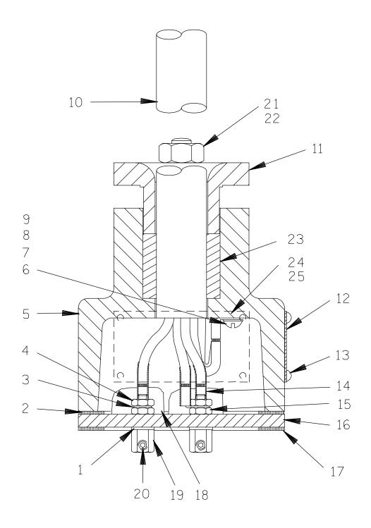
Figure C-3. Terminal Housing And Cable Assembly All-SST Models Only
