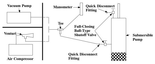
Figure C-8. Vacuum Test System
