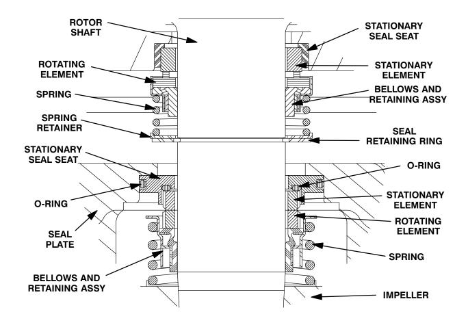
Figure C-4. Upper And Lower Seal Assemblies
