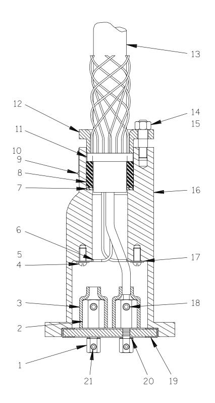
Figure C–2. Terminal Housing And Cable Assembly
