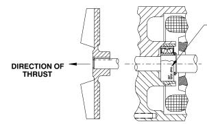
PART NUMBER MARKINGS ARE LOCATED EITHER ON BEARING O.D. (OFFSET FROM CENTER) OR ON SIDE FACE OF BEARING. FOR EITHER TYPE, POSITION BEAR-ING WITH TEXT <u>AWAY FROM</u> IM-PELLER.
