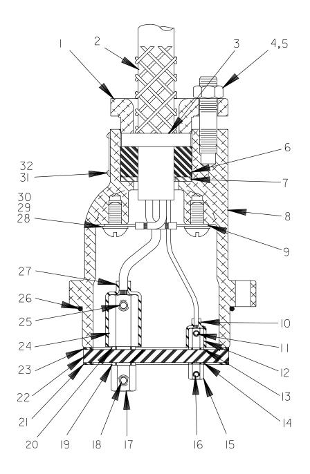
Figure C-2. Model S4F Terminal Housing And Cable Assembly
