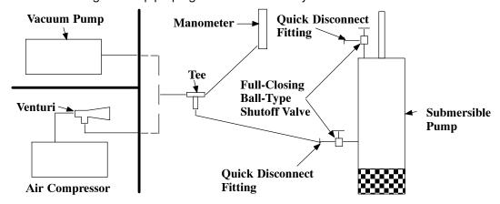
Figure C-8. Vacuum Test System
