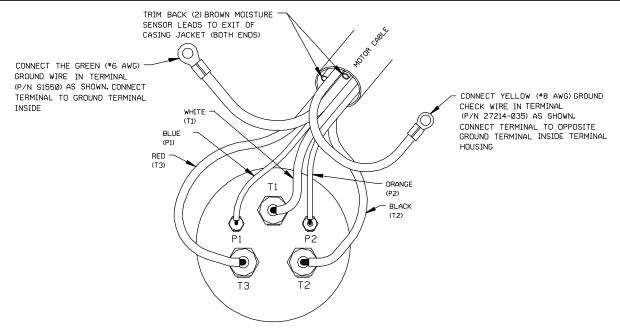
Figure C-6. Terminal Housing Wiring Connections
