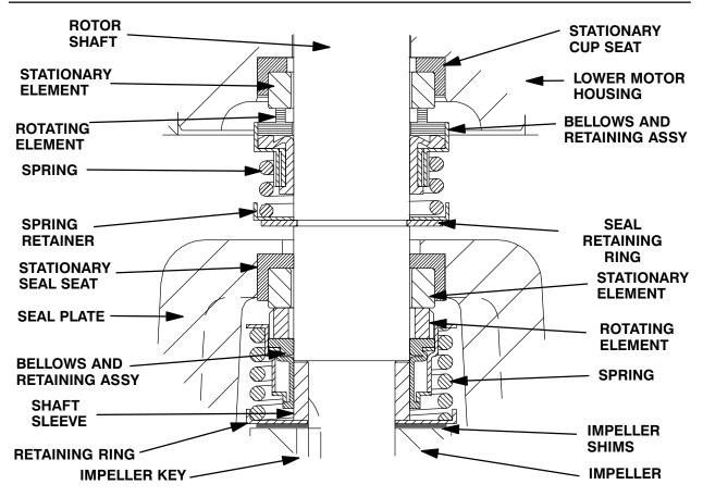
Figure C-4. Upper And Lower Seal Assemblies
