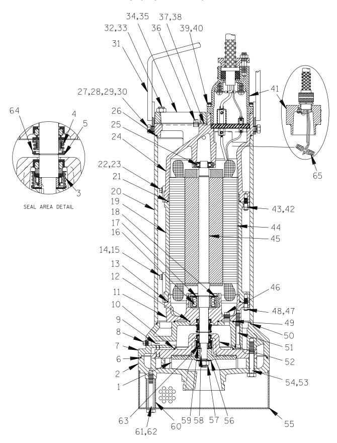
Figure C-1. Typical S4F And S4K Series Pump Assembly
