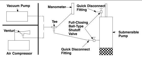
Figure C-10. Vacuum Test System
