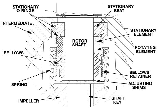
Figure C–4. Lower Seal Assembly
