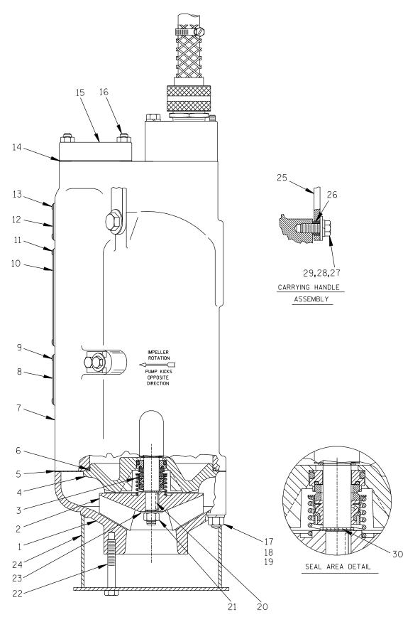
Figure C–1. Typical SM2E Series Pump Assembly
