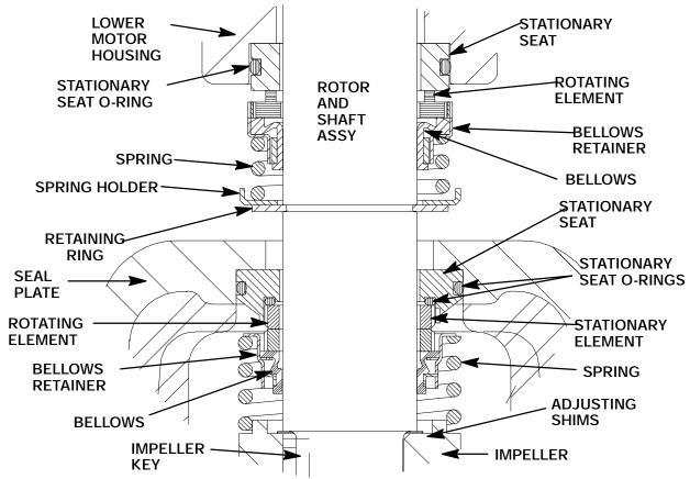
Figure C-3. Upper And Lower Seal Assemblies
