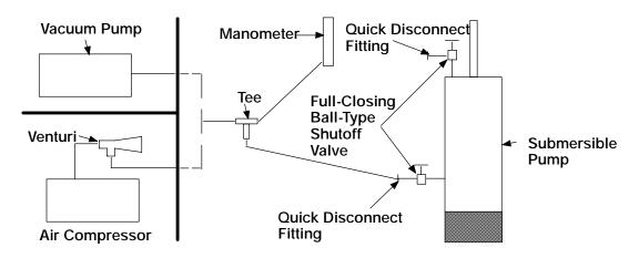
Figure C-8. Vacuum Test System
