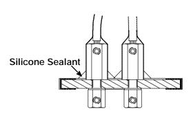
Figure C-7. Silicone Adhesive Sealing
