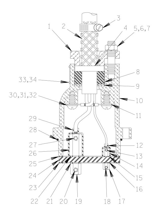
Figure C-2. SM4G's And SM4J's Terminal Housing & Cable Assembly
