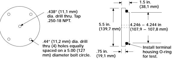
Figure C-9. Motor Vacuum Test Plate
