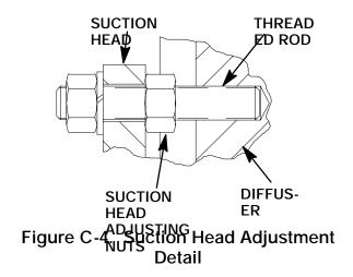
Reach through the suction head opening with a feeler gauge and measure the impeller face clearance. For maximum performance the clearance between the suction head and the impeller should be between 0.010 and 0.015 inch (0,25 and 0,38
