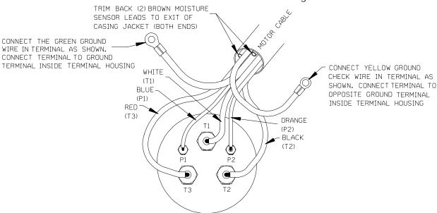
Figure C-6. Terminal Housing Wiring Connections
