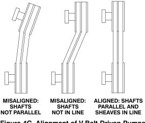
Figure 4C. Alignment of V-Belt Driven Pumps
