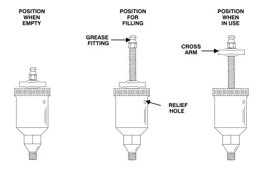
Figure E-4. Automatic Lubricating Grease Cup
