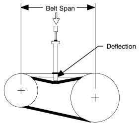
Figure 5. Belt Tension Measurement
