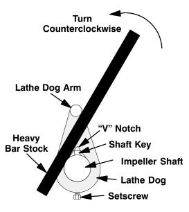
Figure E-2. Loosening Impeller
