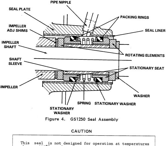
This seal is not designed for operation at temperatures above 110°F. Do not use at higher operating temperatures.
