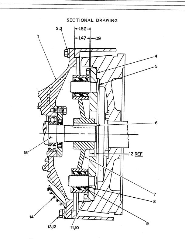
Figure 3. Drive Assembly For Pump Model 14C2-F3L
