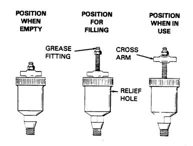
Figure 5. Automatic Lubricating Grease Cup
