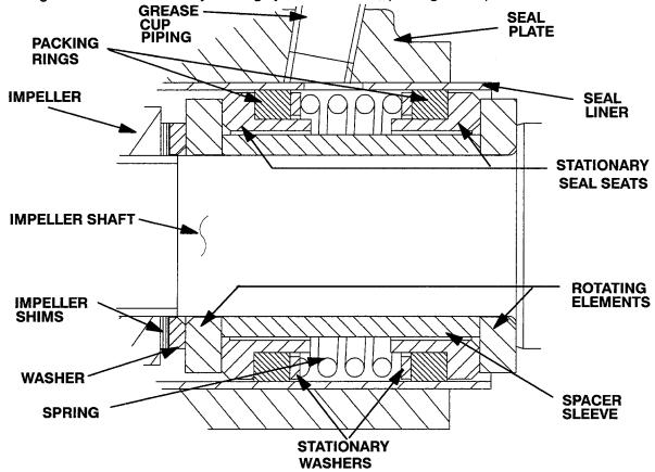
Figure E-4. GS1250 Seal Assembly
