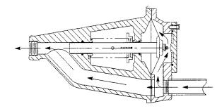
Figure 3. Valve in Open Position
