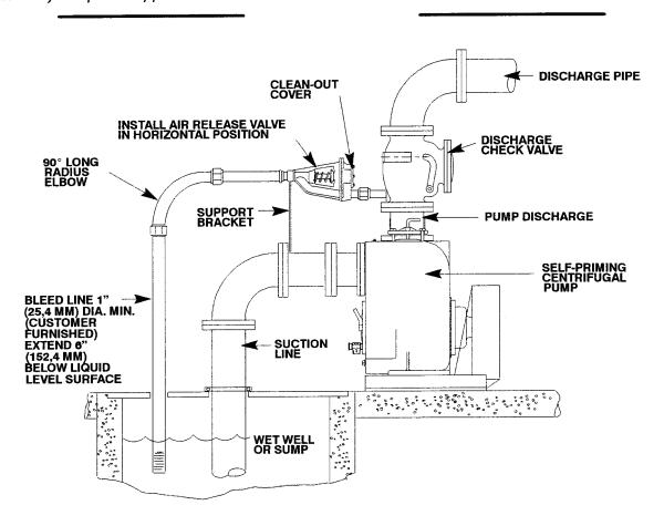
Figure 5. Typical Automatic Air Release Valve Installation
