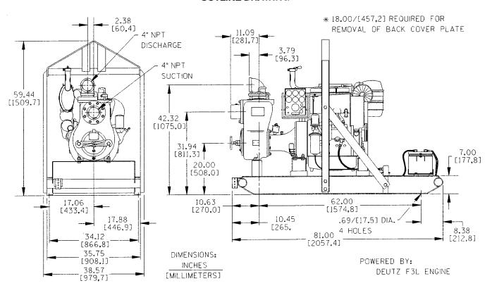
Figure 1. Pump Model 14C2-F3L
