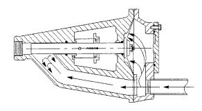
Figure 4. Valve in Closed Position
