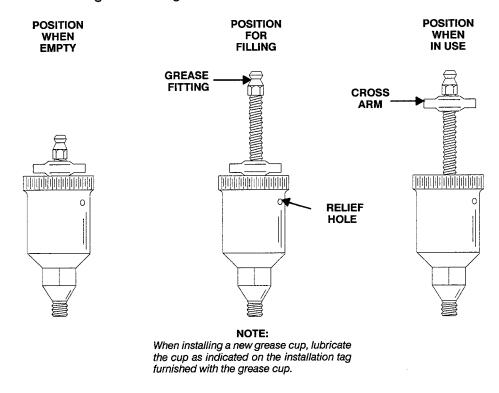
Figure E-5. Automatic Lubricating Grease Cup
