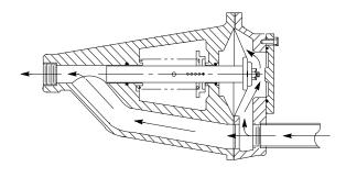
Figure 4. Valve in Open Position
