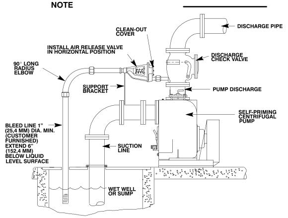
Figure 6. Typical Automatic Air Release Valve Installation
