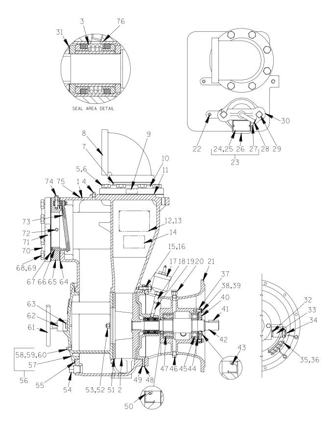
Figure 2. 16C2-(SAE 4/10) Pump End Assy
