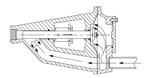
Figure 5. Valve in Closed Position
