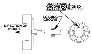
INSTALLATION OF NEW DEPARTURE OR BCA/FEDERAL MOGAL 5300W SERIES BEARINGS (OPEN OR ENCLOSED IMPELLERS) the shaft, it is recommended that bearings be cleaned and inspected **in place**. It is **strongly** recommended that the bearings be replaced **any** time the shaft and bearings are removed.
