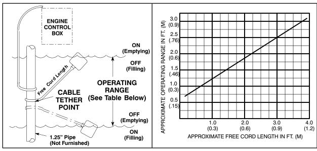
Figure 3. Float Switch Data
