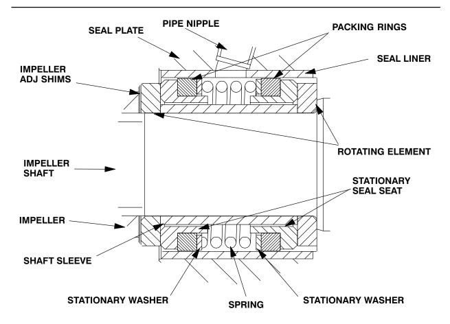
Figure 5. GS1500 Seal Assembly
