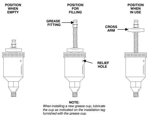
Figure 6. Automatic Lubricating Grease Cup
