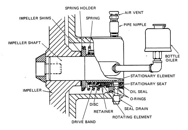
Figure 2. 12461 Seal Assembly
