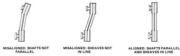
Figure 5C. Alignment of V-Belt Driven Pumps
