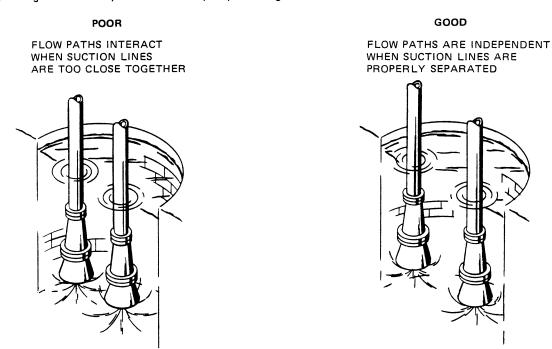
Figure 3. Using Two Pumps in the Same Sump
