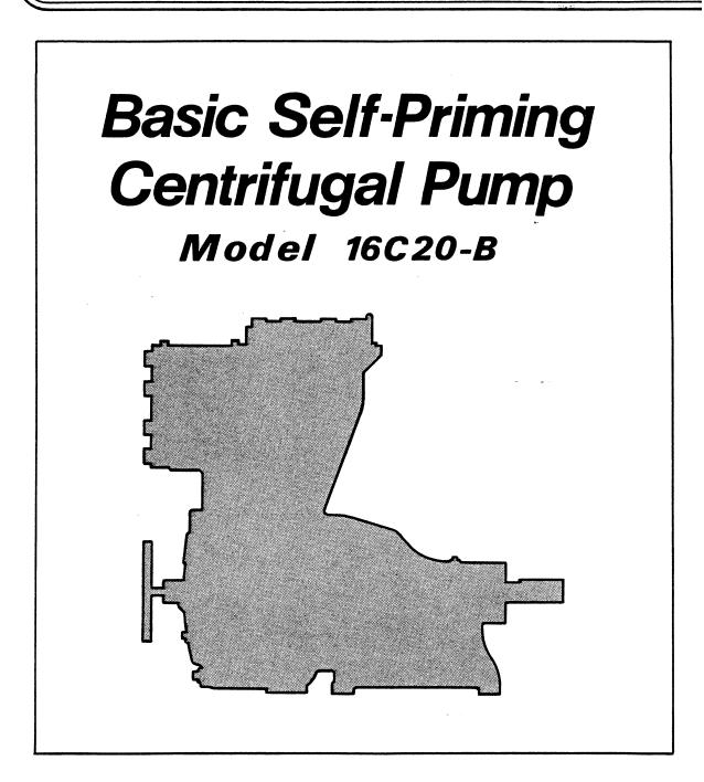
The only moving parts of this pump are the impeller, seal rotating elements, and the shaft. The wear plate, impeller, and seal, which receive the most wear, are easily accessible and can be replaced by removing the cover without disturbing the volute casing and piping. Maintenance and replacement of these three parts will maintain the peak operating efficiency of the pump.
