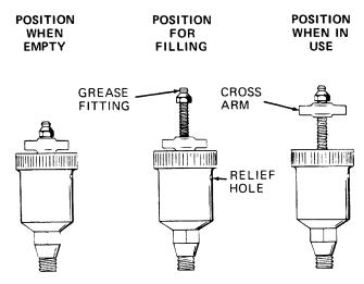
Figure 3. Automatic Lubricating Grease Cup
