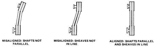
Figure 5C. Alignment of V-Belt Driven Pumps
