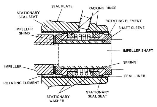
Figure 2. GS-750 Seal Assembly
