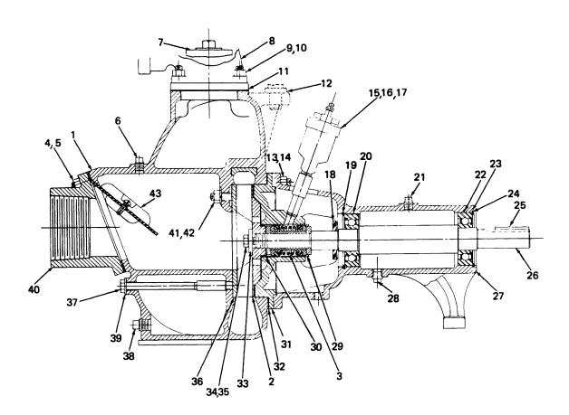
Figure 1. Pump Model 83A2-B
