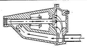
Figure 2. Valve in Closed Position
