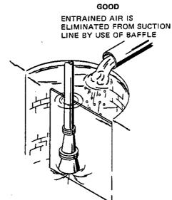
Figure 2. Eliminating Entrained Air Caused by a Fill Pipe
