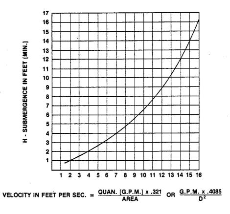
Figure 1. Recommended Minimum Suction Line Submergence Vs. Velocity
