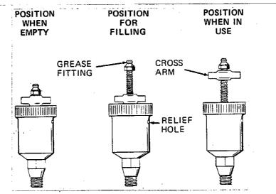
Figure 3. Automatic Lubricating Grease Cup
