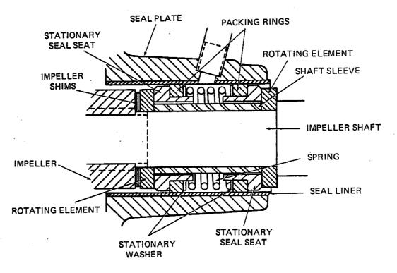
Figure 2. GS-1000 Seal Assembly
