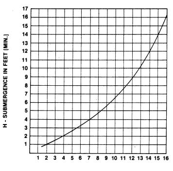
VELOCITY IN FEET PER SEC. =  $\frac{\text{QUAN. [G.P.M.] x .321}}{\text{AREA}}$  OR  $\frac{\text{G.P.M. x .4085}}{\text{D}^2}$
