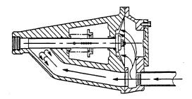
Figure 2. Valve in Closed Position
