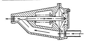
Figure 1. Valve in Open Position
