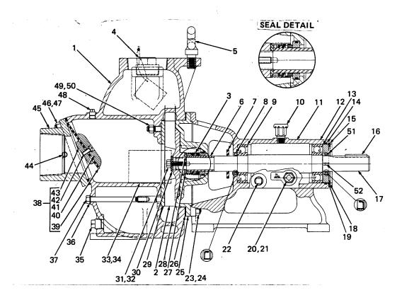
Figure 1. Pump Model 83B52-B
