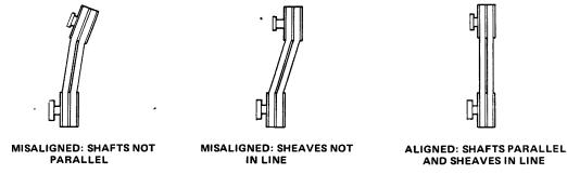
Figure 5C. Alignment of V-Belt Driven Pumps
