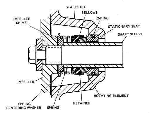
Figure 2. 25284-951 Seal Assembly
