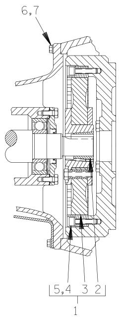
Figure 3. Drive Assembly For Pump End 86A2-(SAE 4/10)
