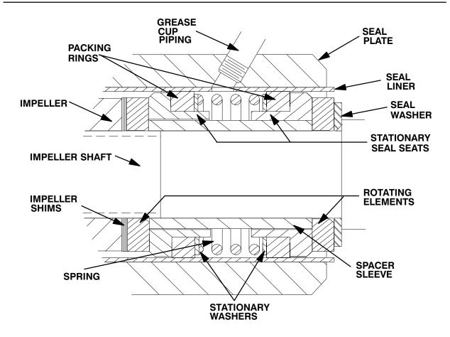
Figure 4. GS1250 Seal Assembly
