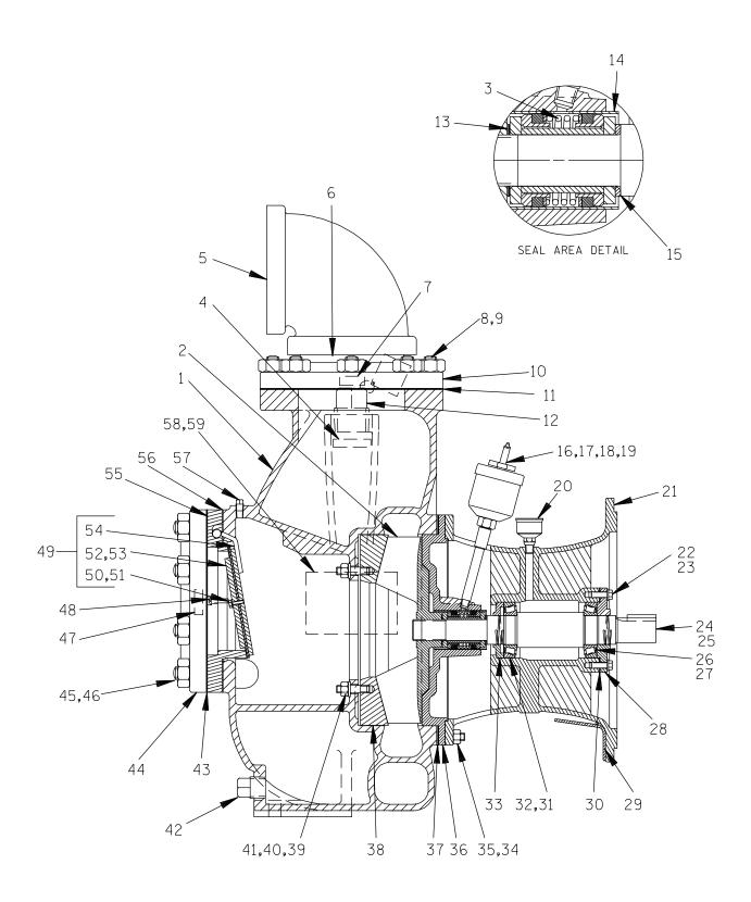
Figure 2. Pump End Assembly 86A2-(SAE 4/10)
