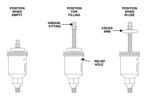
Figure 5. Automatic Lubricating Grease Cup
