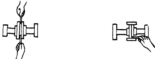
Figure 5A. Aligning Non-Spider Type Couplings
