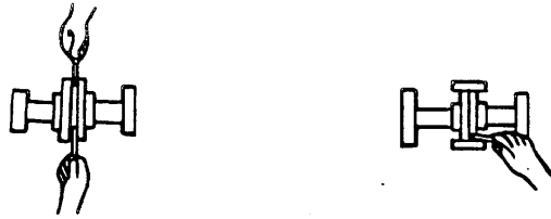
Figure 3B. Aligning Non-Spider Type Couplings
