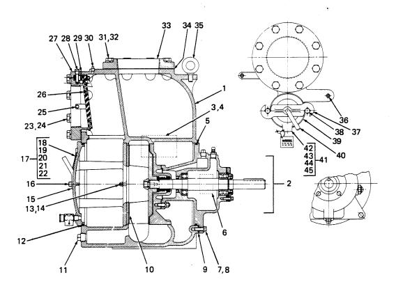
Figure 1. Pump Model T6A3-B
