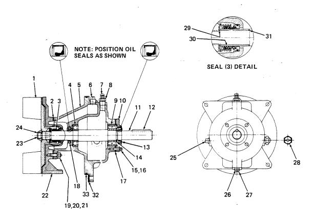
Figure 2. Rotating Assembly for Pump Model T6A3-B
