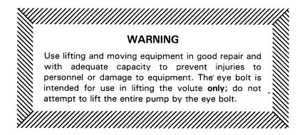
Make sure that hoists and other lifting equipment are of sufficient capacity to safely handle the pump assembly. If chains or cables are used, make certain that they are positioned so that they will not damage the pump, and so that the load will be balanced.
