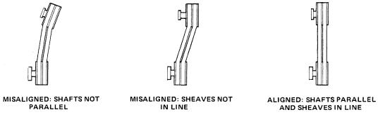
Figure 5C. Alignment of V-Belt Driven Pumps
