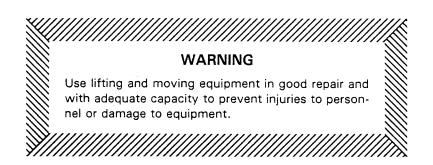
Make sure that hoists and other lifting equipment are of sufficient capacity to safely handle the pumping assembly. If chains and cables are used in lifting, make certain that they are positioned so that they will not damage the pump, and so that the load will be balanced.
