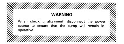
Before checking alignment, tighten the foundation bolts, pump casing and/or pedestal feet, and power source mounting bolts. Make sure that the pump is level.
