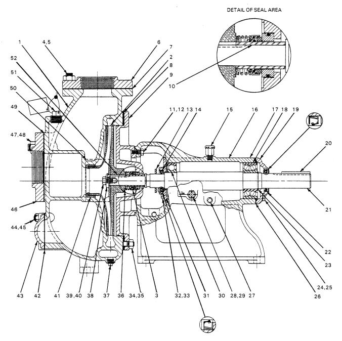
Figure 1. Pump Model 03A52-B
