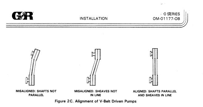
Tighten the belts in accordance with the belt manufacturer's instructions. If the belts are too loose, they will slip; if the belts are too tight, there will be excessive power loss and possible bearing failure. Select pulleys that will match the proper speed ratio; overspeeding the pump may damage both pump and power source.
