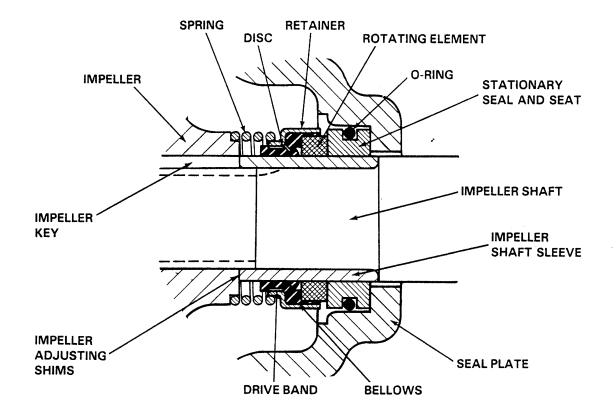
Figure 2. 25284-951 Seal Assembly
