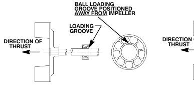
INSTALLATION OF NEW DEPARTURE OR BCA/FEDERAL MOGAL 5300W SERIES BEARINGS (OPEN OR ENCLOSED IMPELLERS)
