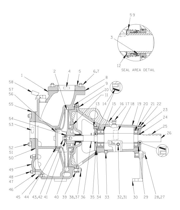
Figure 1. 04B52-B Pump Model Assembly
