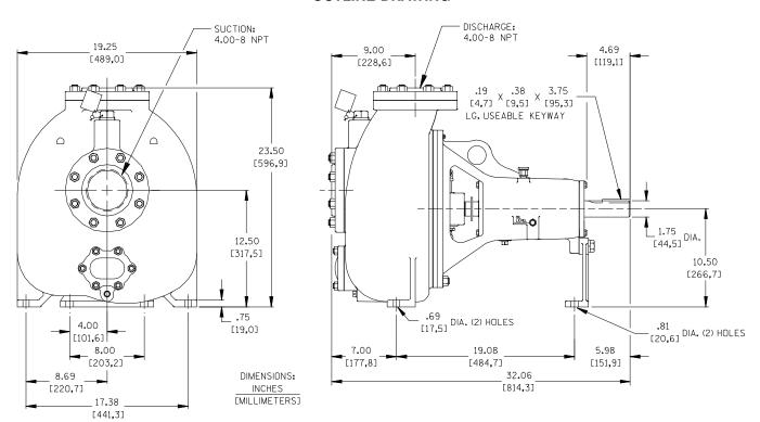
Figure 1. Pump Model 04B52-B
