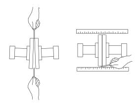
Figure 3B. Aligning Non-Spider Type Couplings
