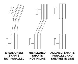
Figure 3C. Alignment of V-Belt Driven Pumps
