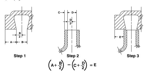
Figure 4. Centering Impeller Within Volute Scroll
