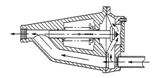
Figure 3. Valve in Open Position
