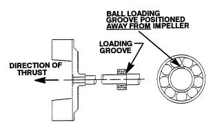
INSTALLATION OF NEW DEPARTURE OR BCA/FEDERAL MOGAL 5300W SERIES BEARINGS (OPEN OR ENCLOSED IMPELLERS)
