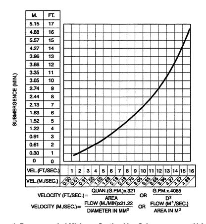
Figure 1. Recommended Minimum Suction Line Submergence vs. Velocity
