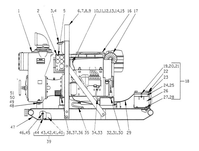
Figure 1. 16C20-F4L Pump Assembly
