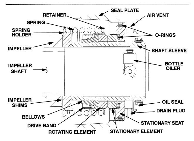
Figure 5. 12461 Seal Assembly
