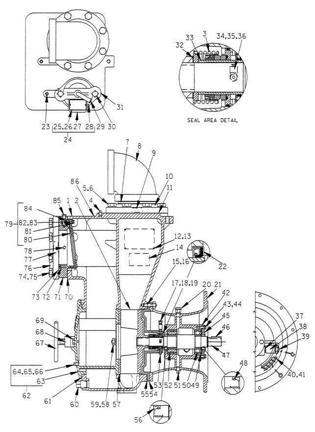
Figure 2. 16C20-(SAE 4/10) Pump End Assembly
