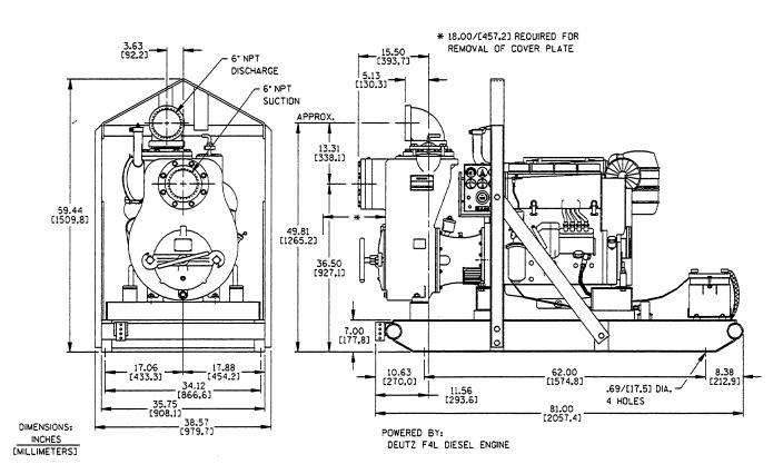
Figure 1. Pump Model 16C20-F4L
